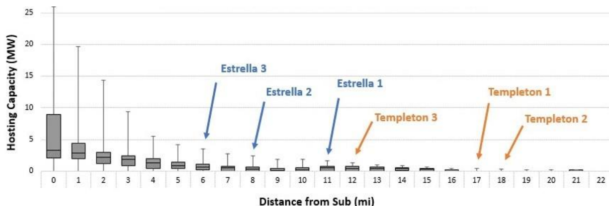
Figure 9. Circuit DER Hosting Capacity versus Distance from Substation
